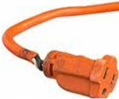
Exposed internal conductors.
