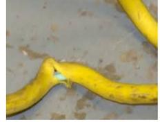
Damaged external insulation
